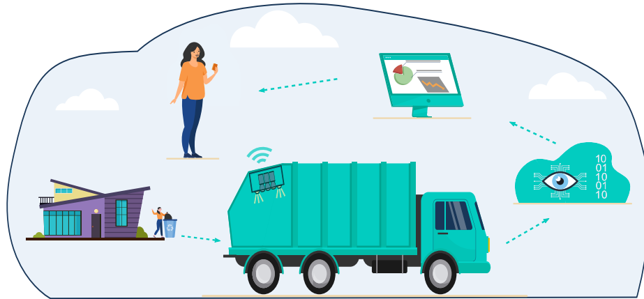
Fig. 1. System overview. In the center of the waste monitoring system is the intelligent garbage truck that is equipped with a complex hardware set combined within a compact and sealed casing. The truck acquires images and sends them for processing to the cloud using a GSM module. After that, the AI model classifies the waste and calculates a waste distribution that is sent to the customer web portal, where the information is communicated to single households. (This figure has been created using and modifying resources from https://www.freepik.com/pch-vector .)
