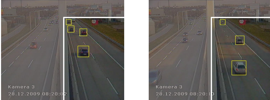
Figure 23: Sample detections on the first highway sequence. Since we trained our detectors with patches showing the rear end of cars, we evaluate our classifiers only on the right lane. The white box shows the boundaries of the detection region.
