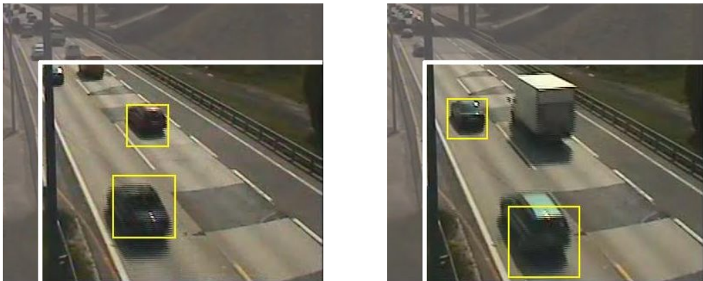
Figure 26: Sample detections on the second highway sequence. The white box shows the boundaries of the detection region.
