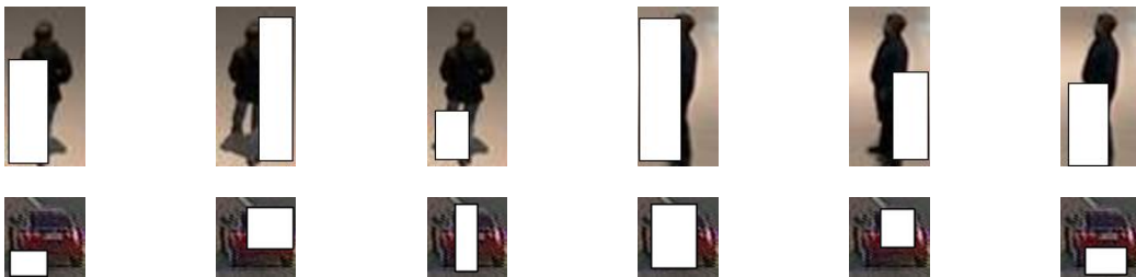
Figure 14: Visualisation of locations of selected HOG features. These features concentrate on areas with highly discriminative edges, such as feet and contour information of the torso for human detection and distinctive silhouette edge structures for car detection.
